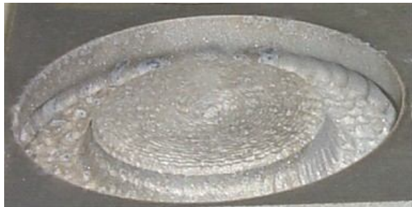
Figure 2 – Milling with Abrasive Waterjet
