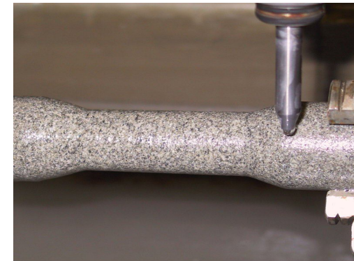
Figure 3 – Turning with Waterjet
